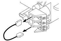
Figure 36 - Connecting Wall Switch to Control Cover
